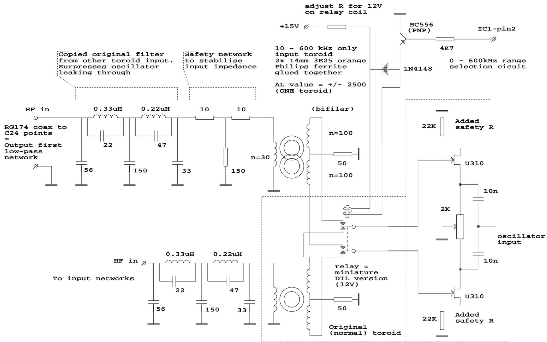
Input filter, toroid and relay on a small piece of board, placed on the solder side of the Rx board. Make mixer input wiring as short and compact as possible. DON'T blow your mixer FET's during soldering !!
